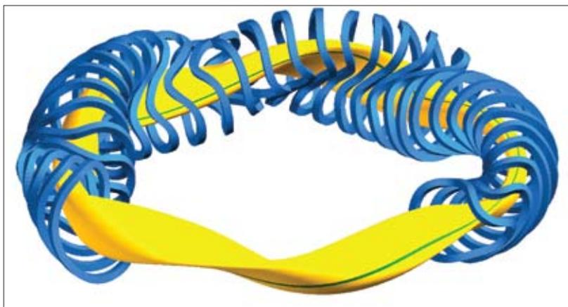
Figure 11 (right): Schematic arrangement of a magnetic field coil system for the Wendelstein 7-X stellarator under construction in Greifswald, Germany. Source: Max Planck Institute.
