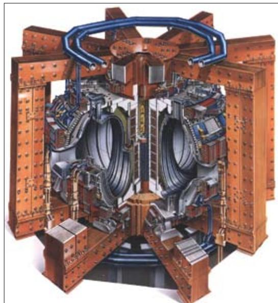
Figure 7: The JET tokamak. Source: EDF/JET.
